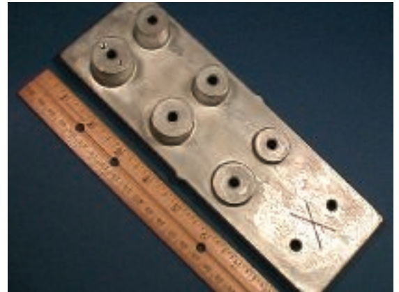
Top side of test panel before finishing and corrosion testing
