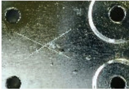
Blisters formed on "dual nickel" Cu/Ni/Cr plate after three month exposure
