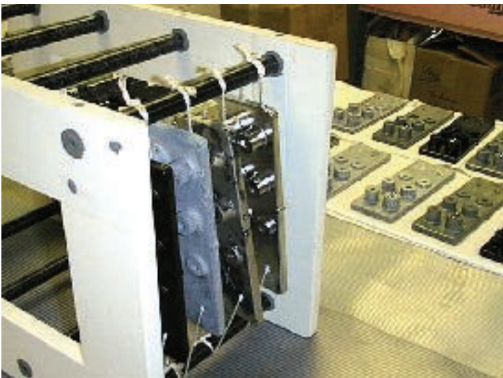
Test rack and panels outside humidity chamber
